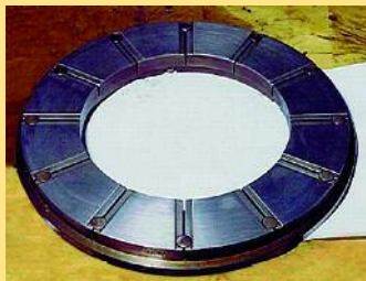
After 30,000 running hours on Shell Turbo Oil GT 32
